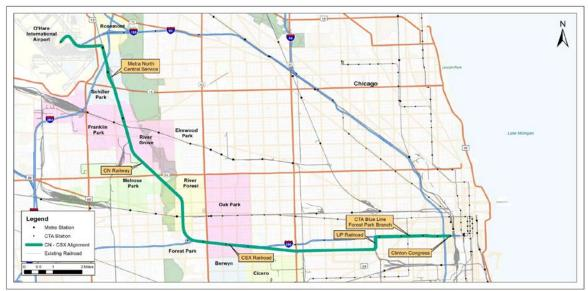
The CSX-CN mainline corridor offers the potential for exclusive or near exclusive track use from Junction B-12 to Rockwell Street. There are 11 at-grade street crossings, but they all have gates and signals in place. There are also 28 structures carrying the railroad over a street, and 2 structures carrying the railroad over the Des Plaines River and small stream near the CN Schiller Park Yard (the condition of these structures is
